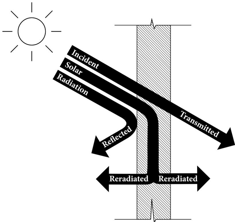
Figure 31 – Components of the Solar Load on a given surface. Source: redrawn by the Author
